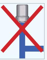
In locating the water hammer arrester on the systemit is important to avoid creating areas where stagnant water may collect, i.e. situations where bacterial colonies can proliferate. For example, installation at the top of a riser can create areas with still water ("dead zones"), even though the water hammer arrester will function properly. Consequently, this kind of installation must be avoided.
