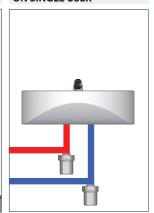
The water hammer arrester can be installed in vertical, horizontal or inverted positions
